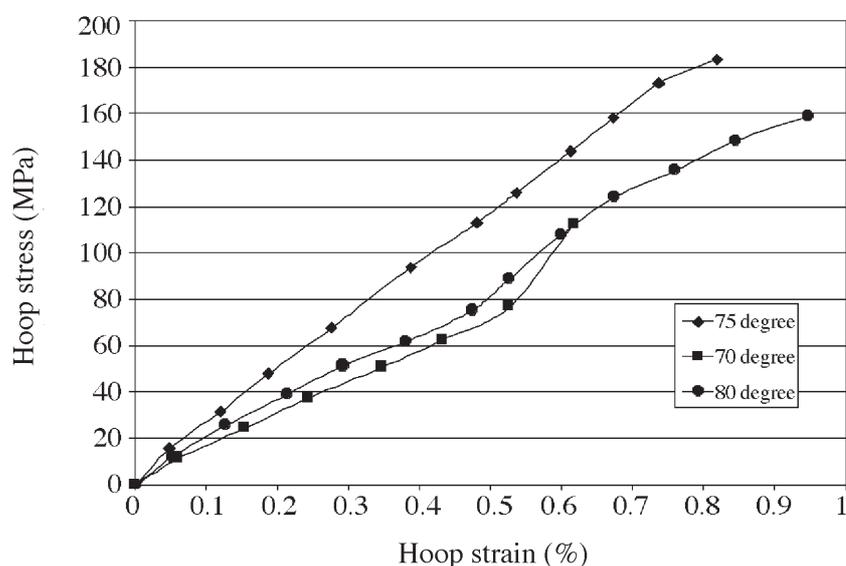
**Figure 8. Hoop stress versus hoop strain for different winding angles under loading mode (II)**
