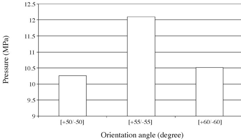
Figure 6. Pressure versus orientation for composite tube under loading mode (III)
