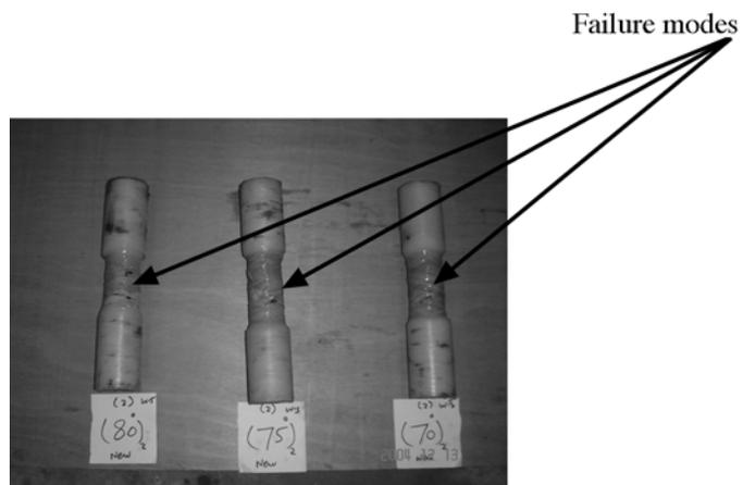
**Figure 11. Samples of composite tubes failed under loading mode II**
