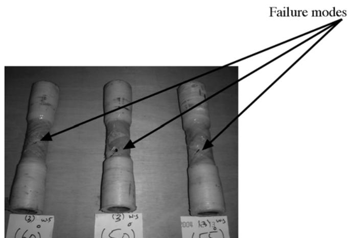
**Figure 12. Samples of composite tubes failed under loading mode III**
